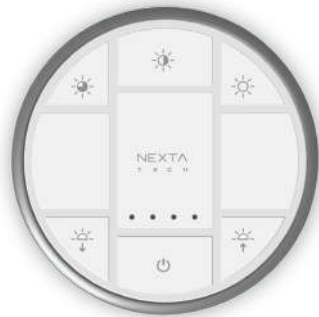
HB80-1DIM Radio control, rolling code 433.92 MHz, 1 channel, On-Off function, dimmer up/down, select intensity, 30%-60%-100%. CR2450 battery.
