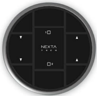
HB80-2L Radio control, rolling code 433.92 MHz, 2 channels, On-Off function,dimmer up/down, open-close-stop(motor). CR2450 battery.
