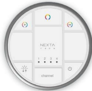
HB80-4C Radio control, rolling code 433.92 MHz, 4 channels + All, On-Off, dimmer up/down, colour control RGB/RGBW and CCT, dynamic cycle control. CR2450 battery.
