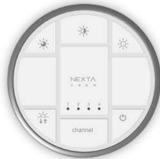
HB80-4DIM Radio control, rolling code 433.92MHz, 4channels + All, On-Off , dimmer up/down, select intensity, 30%-60%-100%. CR2450 battery.
