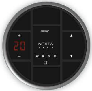
HB80-30RGBW Radio control, rolling code 433.92 MHz, 30 channels, On-Off, dimmer up/down, colour control RGB/RGBW and CCT, dynamic cycle control, open-close-stop (motor). CR2450 battery.
